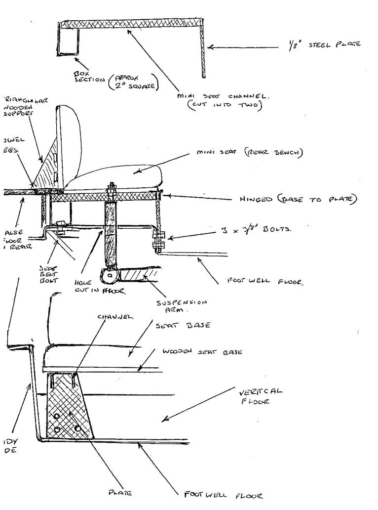
The S/A top mount goes through a hole in the channel, it does stick up about 4" but a hole in the plywood seat base will solve that and it won't cause a sore posterior (the foams thick !!!!).
